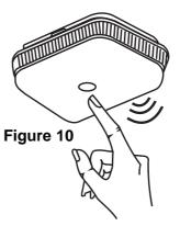
When you press the test button it simulates the effect of smoke during a real fire. So, there is no need to test the Alarm with smoke.
